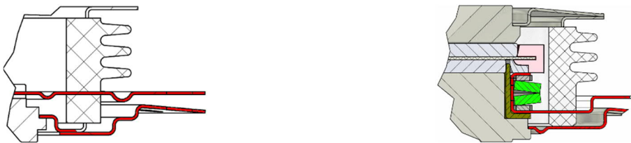
Figure 2: Cross-sections of the gate-lead bushing of the earlier (left) and new (right) IGCT housing platform. The red parts show the current paths through the hermetic housing. ABB Switzerland Ltd is an owner of the design patents for both IGCT housing platforms.
