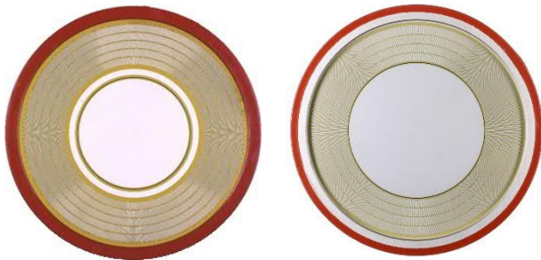
Figure 1: Left: The conventional RC-IGCT wafer with the gate contact in the separation between diode- and GCT parts. Right: The newly developed RC-IGCT wafer with the outer ring gate contact.
