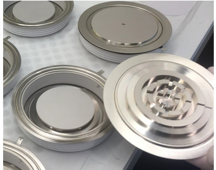
06 Pole piece with expansion volume to contain plasma blast
