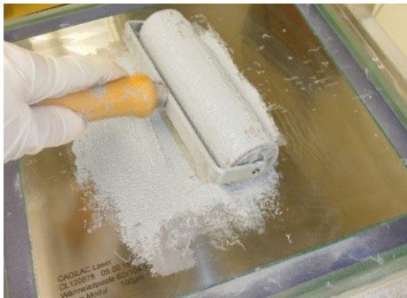
06a Applying the paste onto the stencil using a rubber roller
