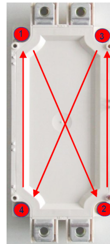
11 Tightening sequence to mount the module to the heat sink
