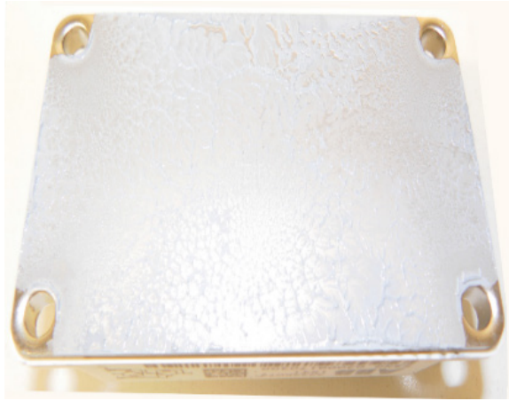
09 Example of good paste coverage
