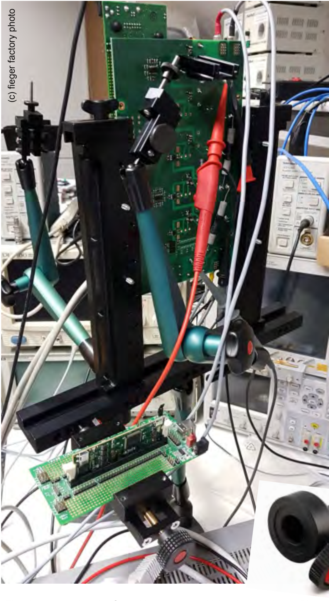
The vice mounted on the ClampMan using an additional base adapter "104500"
