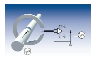
Fig. 1: Principle of the open loop transducer
