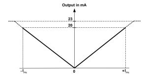
Note: 1) The performance specified in the datasheet is valid within the 0-20 mA output range only.
