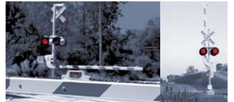
Picture 6: Signaling at a crossing gate
