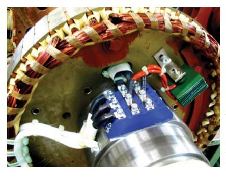
Three phase leg diode modules **PSTKD 82** mounted on the high speed rotating shaft of an UPS System
