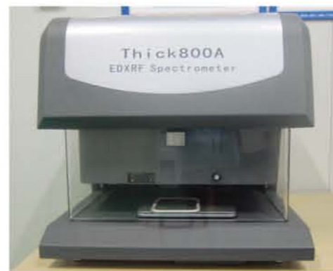
Fluorescence X-ray gauge (Precision: \pm 5\% )
