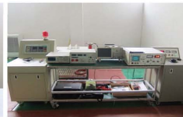
PD and dielectric strength test bench: (Testing range: 0-20kVac/dc)
