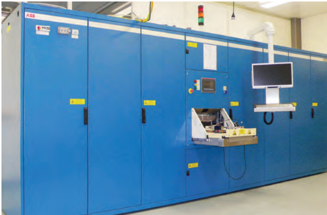
Dynamic IGCT, GTO and diode test system
