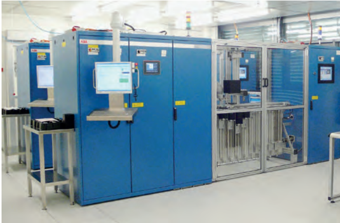
Automated IGBT and diode dies test system
