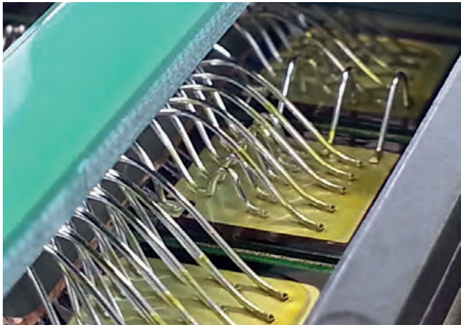
Fig. 5 Stich-bond layout and improved bonding parameters boost the power cycling capability
